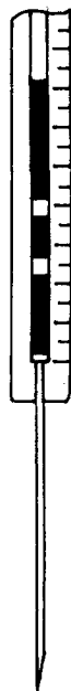
FIG. 1. Syringe-filling technique. Black sections in barrel are solvent or sample solution; clear sections represent air.
